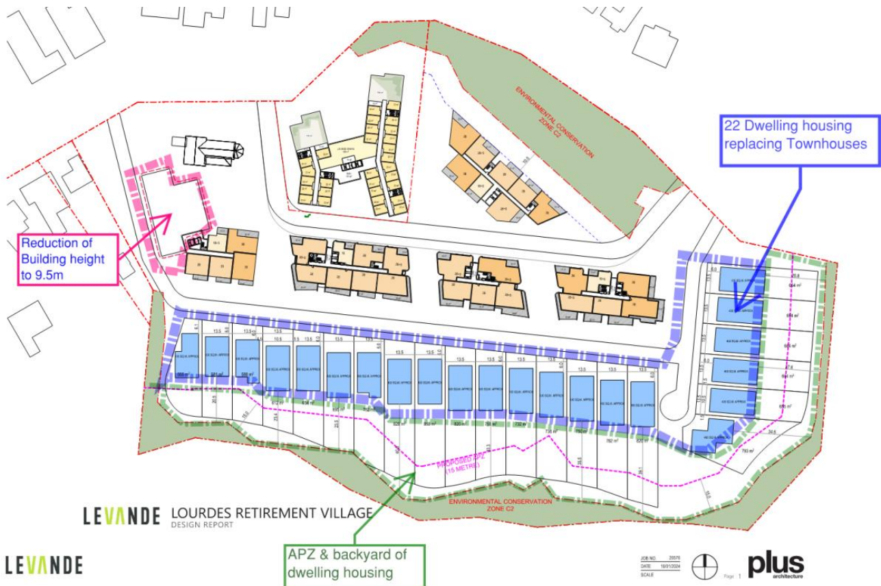
Figure 7 Illustrative Master Plan – revised by proponent following Panel post-exhibition meeting (source: Plus Architecture)
