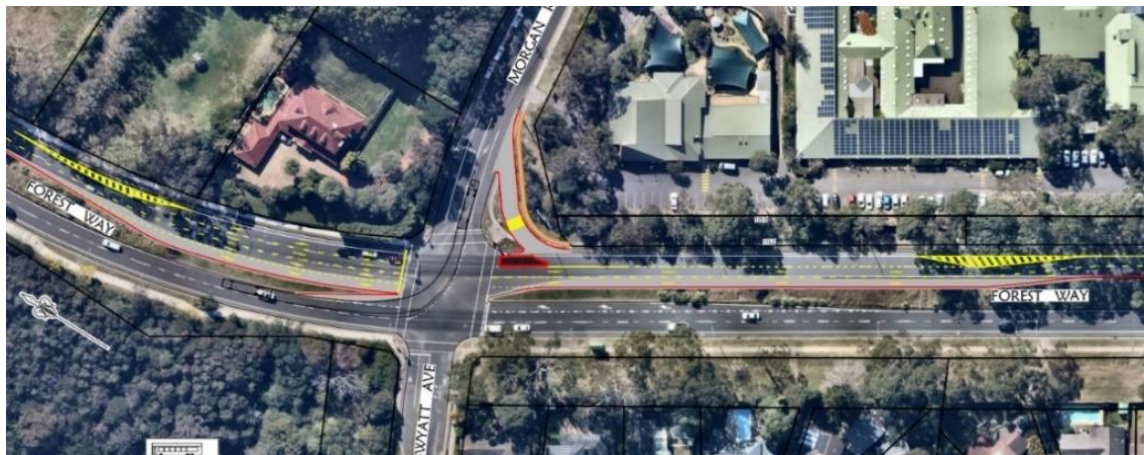
Figure 3.11 – Proposed new slip lane on Forest Way – NOT on land owned by Council
