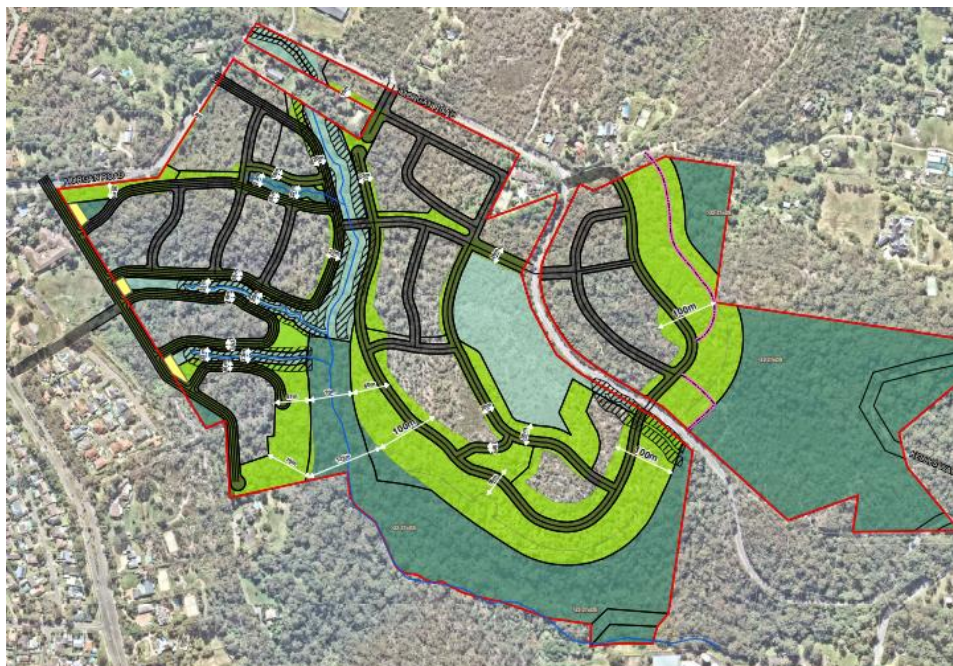
Figure 6.3 – Proposed development design for the PP site showing the extensive asset protection zones
